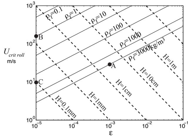
Figure 2: Critical flow speed (from Eq.1) for roll waves versus channel aspect ratio for several fluid densities (solid lines) for constant rock properties of  $\beta = 1$  km/s and  $\rho_s = 2500$  kg/m<sup>3</sup>. Dashed lines indicate crack thickness for  $f \sim U/L \sim 1$  Hz. Points A,B and C refer to conditions discussed in the text.
