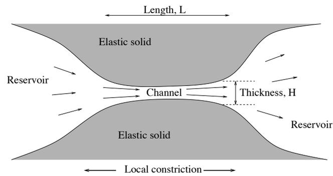
Figure 1: Schematic illustration of a channel between two reservoirs. Flow is driven through the channel by a pressure difference maintained between the reservoirs. The channel is tabular, and its walls deform elastically in response to pressure changes in the fluid.
